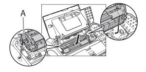
**9** Push the toner cartridge to make sure it is properly set in the machine.
